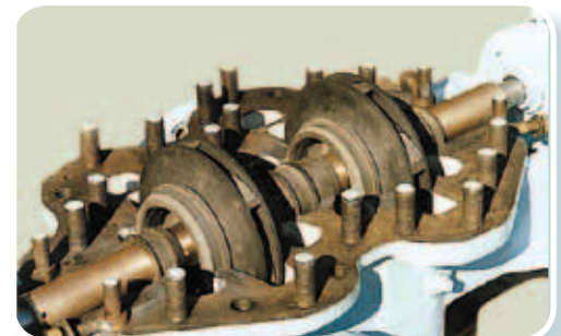
SIMSITE® IMPELLER & RINGS TWO STAGE PUMP FROM SIMSITE® GRADE 300
