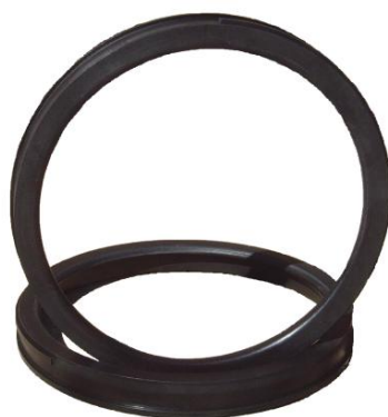
Simsite® Composite Rings are corrosion resistant and wear better than metallic rings. Because they will not seize, or gall like metallic rings, they run with tighter clearances, which increase efficiency and decrease energy consumption.
