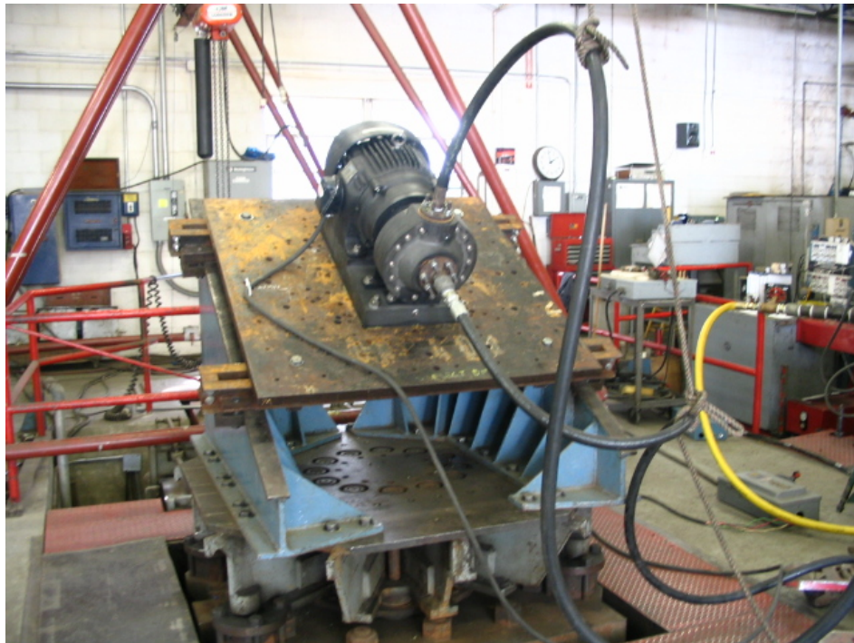
Pump Shaft Parallel to Incline
