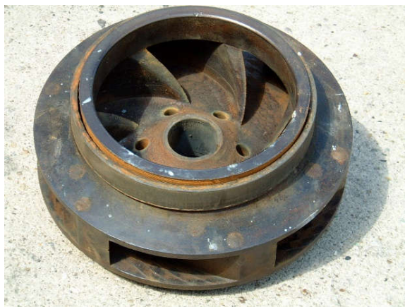
SIMSITE® Impeller and Ring Model 8 x 6 VLM after 10 Years of Continuous S.W. Service
