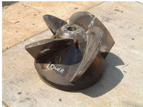
SIMSITE® 36 Hi Flo Impeller, After 18 years of Continuous S.W. Service.
